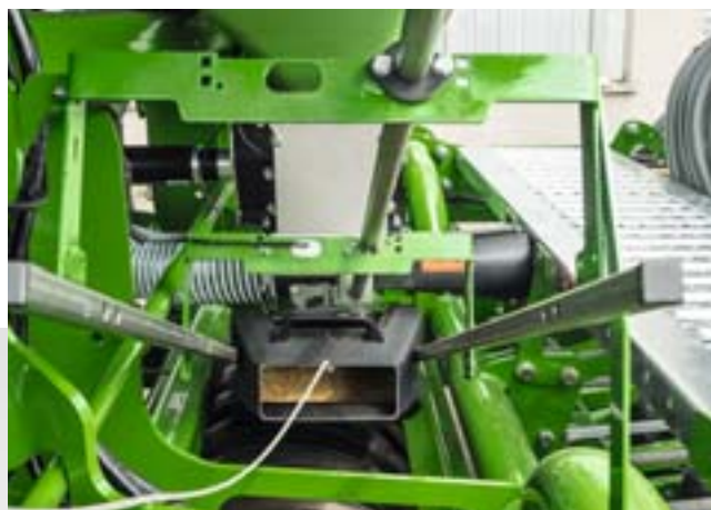
✓ Kalibreringstrug i kalibreringsposition
